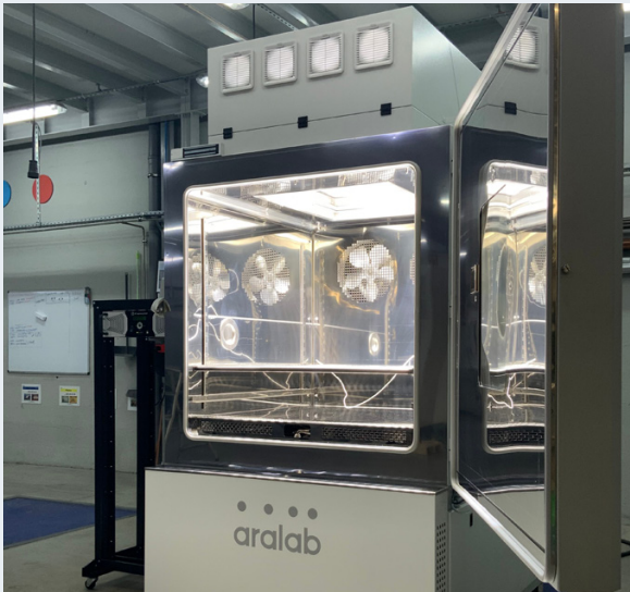
SOLAR AND UV RADIATION CHAMBER
